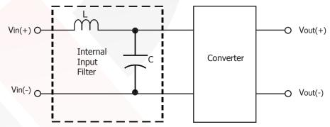
Figure E: Internal Input Filter Diagram
