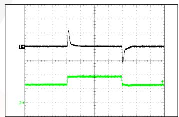
Figure 12: Output voltage response to step-change in input voltage at full load current. Load cap: 100uF electrolytic capacitance. Ch1: Vout (1V/div), Ch 2: Vin (20V/div). Time Scale (1ms/div).
