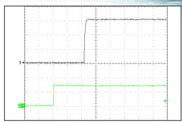
Figure 8: Turn-on transient at full resistive load and zero output capacitance initiated by Vin. ON/OFF Pin previously low. Ch 1: Vout (5V/div). Ch 2: Vin (20V/div). Time Scale (100ms/div).
