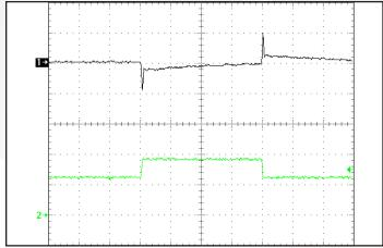
Figure 11: Output voltage response to step-change in load current (50%-75%-50% of lout(max);  $dI/dt = 0.1 \text{ A/\mu s}$ ). Load cap:  $1 \mu F$  ceramic capacitor. Ch 1: Vout (500mV/div), Ch 2: Iout (5A/div). Time Scale (1ms/div).
