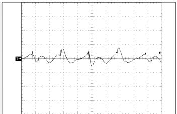
Figure 10: Output voltage ripple, Vout, at nominal input voltage and rated load current (50 mV/div). Load Capacitance: IuF ceramic capacitor. Bandwidth: 20 MHz. Time Scale (2µs/div). See Figure 17.
