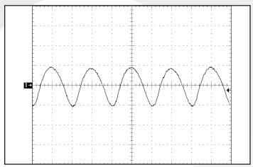
Figure 9: Input terminal current ripple, i<sub>C</sub>, at full rated output current and nominal input voltage with SynQor MCOTS filter module (1 A/div). Bandwidth: 20MHz. Time Scale (2µs/div). See Figure 17.
