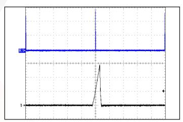
Figure 18: Load current (10A/div) as a function of time (400us/div) when the converter attempts to turn on into a 10 m $\Omega$  short circuit. Reference 1 (40ms/div).
