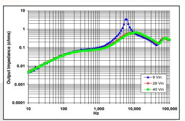
**Figure 13:** Magnitude of incremental output impedance ( $Z_{out} = v_{out}/v_{out}$ ) for minimum, nominal, and maximum input voltage at full rated power.
